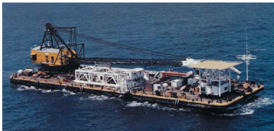
A Taylor welding spread and saturation system on a Brown & Root derrick barge (Collection of Drew Michel)
